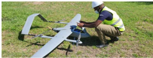
VTOL drone (Vertical Take Off and Landing) Long distance (150km in air) Payload 2kg
